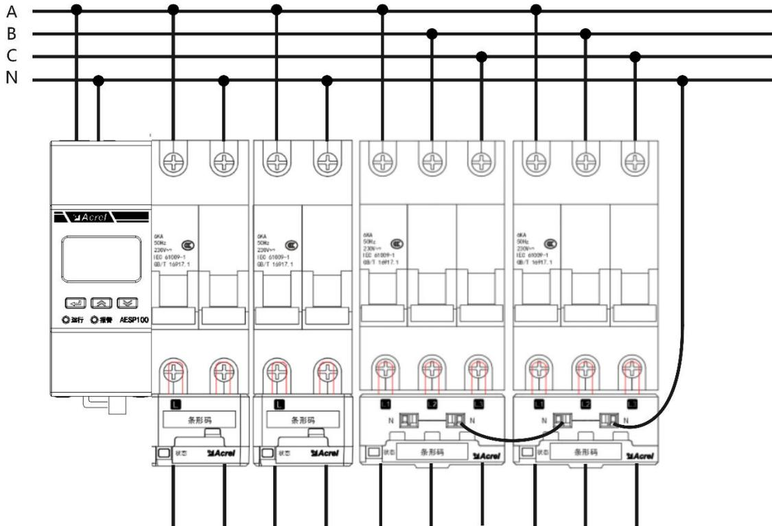
Figure 6. Device installation wiring example diagram
