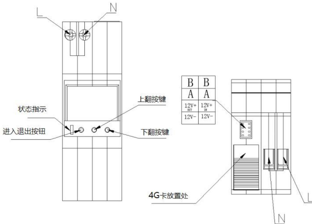
Figure 4. Schematic diagram of the intelligent gateway wiring terminal
