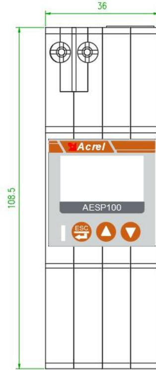
Figure 2. Dimension diagram of the intelligent gateway
