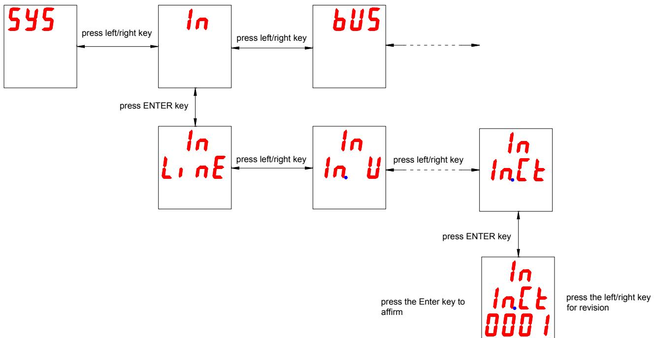
Note: The voltage transformation ratio (In.Pt) setting is similar. Other parameters in this menu need not revision usually.
