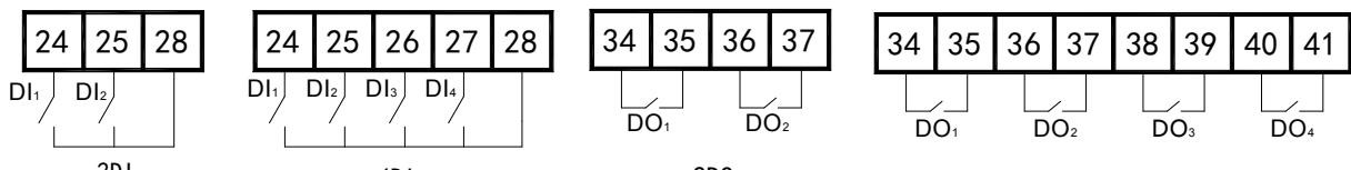
Switch input adopt wet contact switch signal input mode, with built-in +5V operational power supply, the meter need not external power supply. When the external is in ON or OFF, the ON or OFF information is collected by the input module of meter switch and is displaying locally, and implement remote transmission function, i.e. "remote signaling" function by meter digital port RS485.
