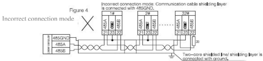
Recommendation of adding matched resistance between A1 B of the last meter, the rated resistance range is 120Ω~10kΩ.
