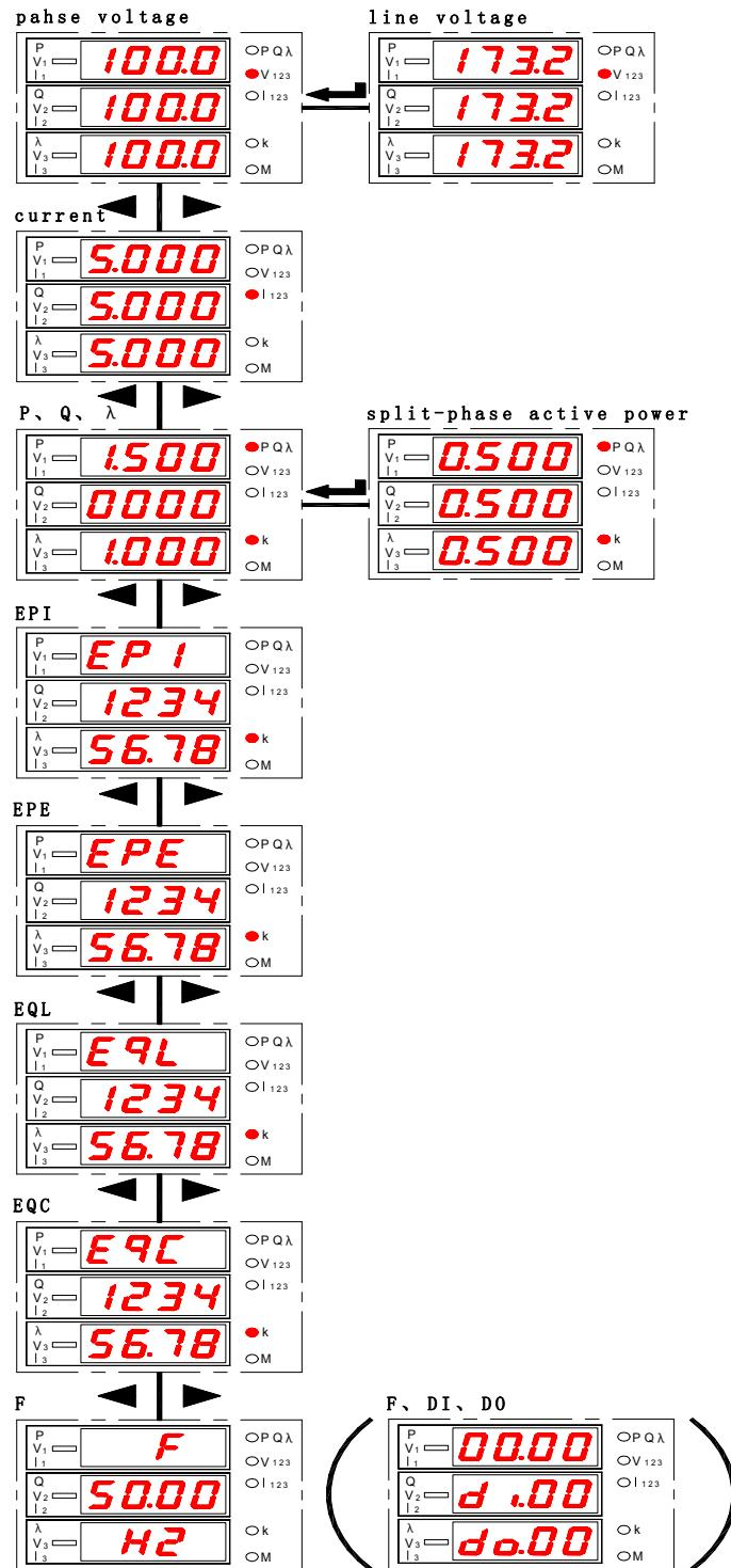
3-phase-4-wire power meter, electric energy meter, electric parameter checking flow chart(LED).
