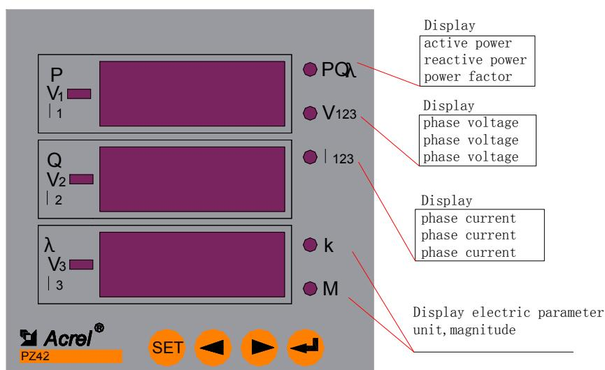
In the right indicators, if only kor M lights, and Level 1 number code display: EPI、EPE、EqL or EqC, then Level 2, Level 3 display :electric energy data: Level 2 is high bits, Level 3 is low bits; if Level 1 display EPI, Level 2 display 0011, Level 3 display 01.58, k indicator lights, other indicators never illuminate, then active electric energy is used (Power Consumption): 1101.58 kWh.
